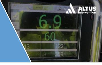
Our new integrated digital recording system offers real-time data measurement of nitrogen flow, pumping pressure, and temperature all from one compact system. This reduces time spent testing by up to 1 hour per test, resulting in significant savings for operators.
